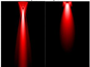
**Figure 9.** Numeric calculations of the reflected sound field based on (21). The source is in the centre of the sphere segment  $\theta_m = \pi/10$ , R=5.4 m. Left: k=18.4,  $kR(1-\cos\theta_m=4.8)$ , Right: k=4.6;  $kR(1-\cos\theta_m)=1.2$
