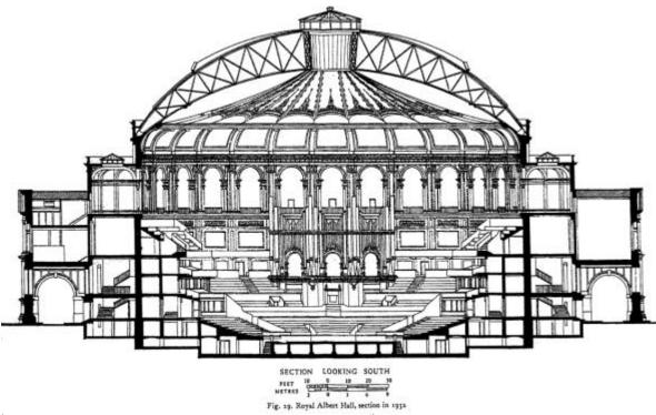
Figure 1 Section of the hall with the original velarium
