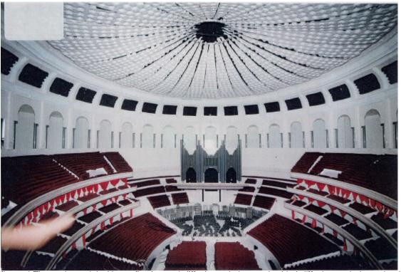
figure 4 The scale model with a reflecting and diffusing velarium and added diffusion and absorption in the cove in the cove
