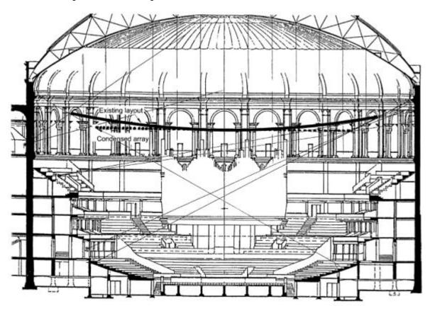
Figure 6. Section of the existing and the new, condensed mushroom array (section)
