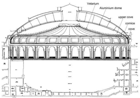
Figure 5. The principle of a acoustically reflecting velarium
