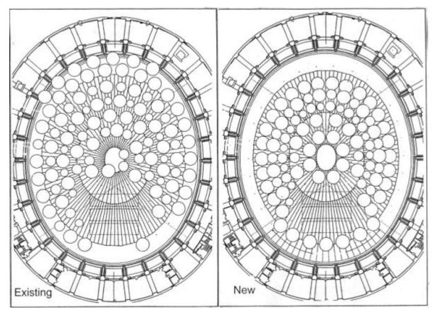
Figure 7 existing and new mushroom array (plan). The finally chosen configuration is slightly more randomised than drawn here.
