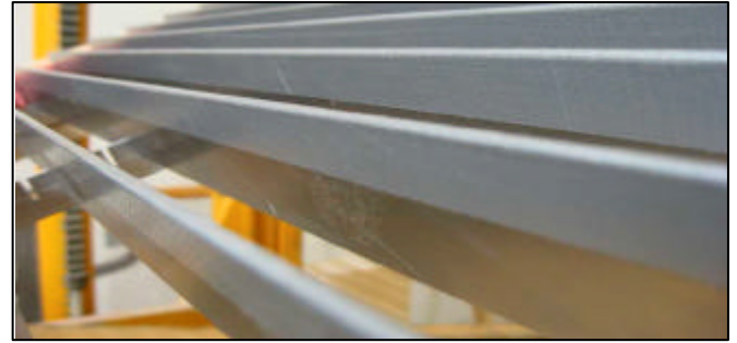
Figure 8: Bearing bars with tape-rounded edges
