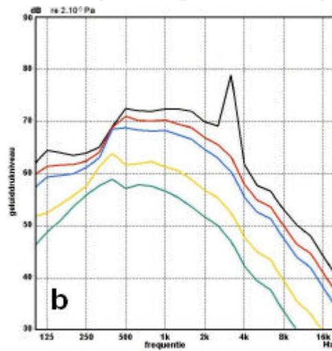
Figure 17a-b: Measurements on the test grating with a bar height of 40 mm with sharp edges (a) and with tape-rounded edges (b).
