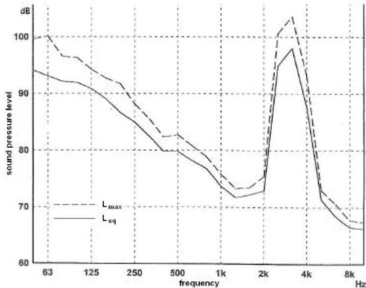
Figure 6: Spectral sound pressure levels of the grating measured in practice
