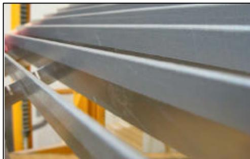
Figure 16: Bearing bars with tape-rounded edges
