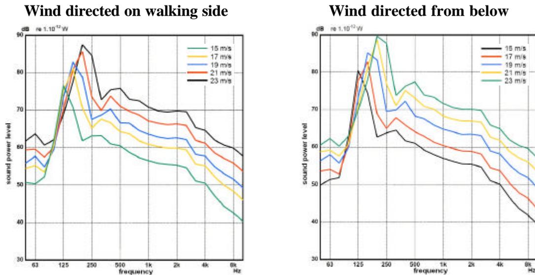
Figure 4: Spectral sound power levels of the grating at different air velocities
