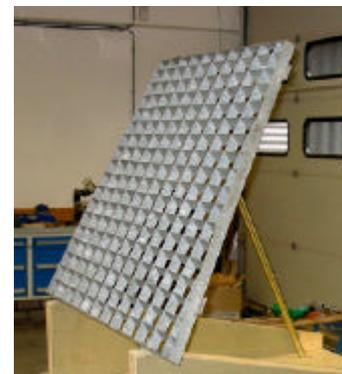
Figure 5: Grating with slightly tilted and non-tilted bars
