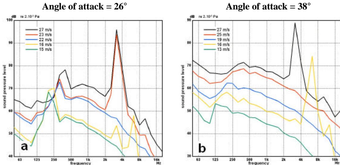
Figure 13a-b: Measurements on the test grating with a bar height of 30 mm and a c.t.c. spacing of 40 mm for two different angles of attack.
