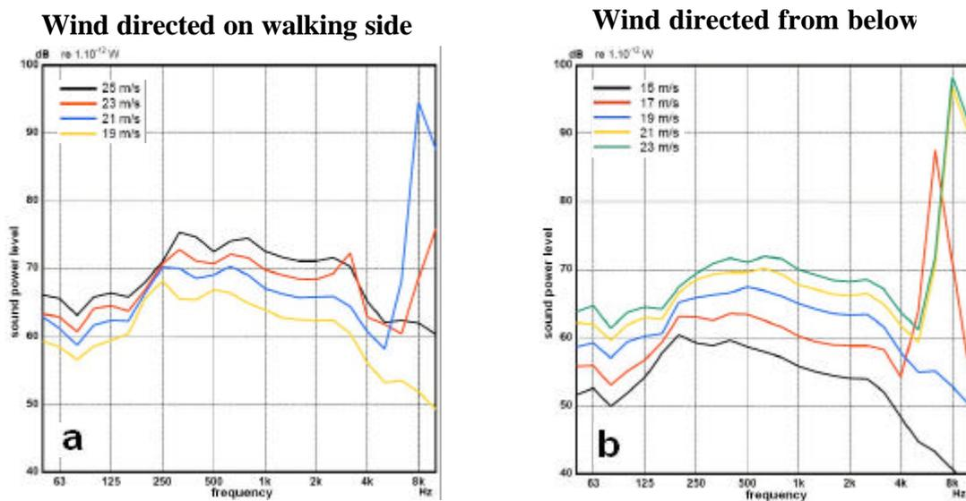
Figure 3: Spectral sound power levels of the grating at different air velocities
