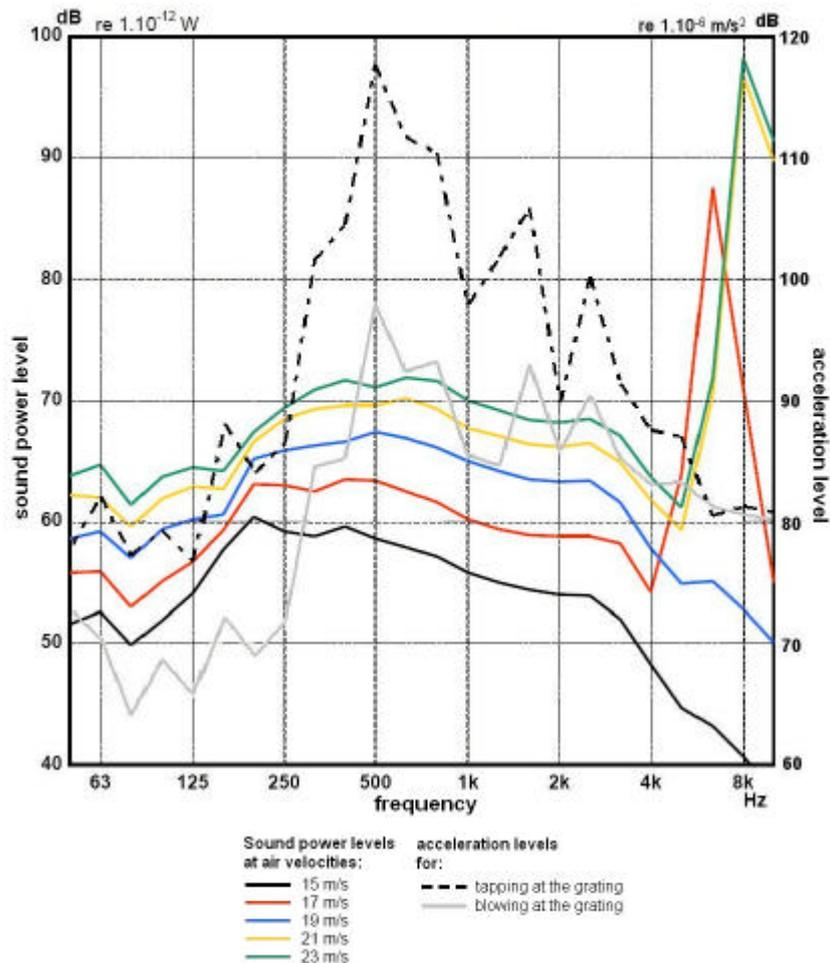
Figure 8: Spectral sound power levels and acceleration levels of grating 1 of building 1
