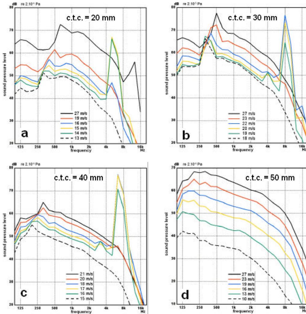
Figure 14a-d: Measurements on the test grating with a bar height of 20 mm.
