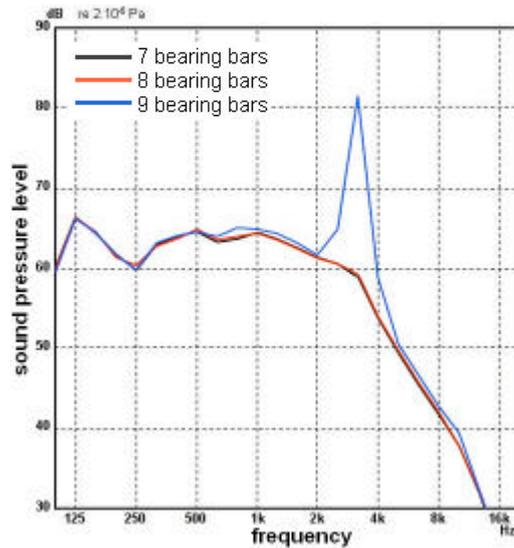
Figure 15: Dependency of number of bearing bars
