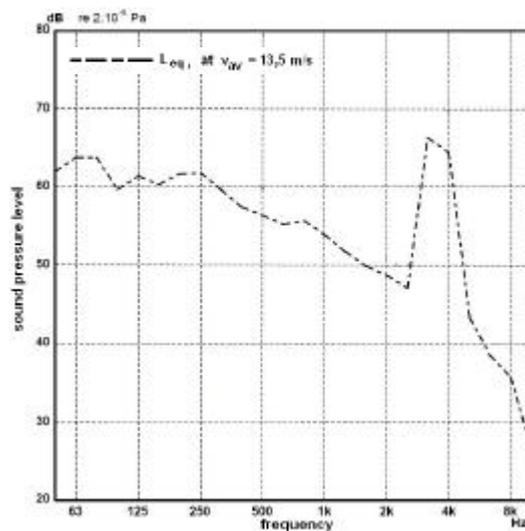
Figure 7: Spectrum of sound level of grating in practice at a distance of about 80 meters. The high sound levels up to a frequency of 500 Hz are due to high wind speeds.
