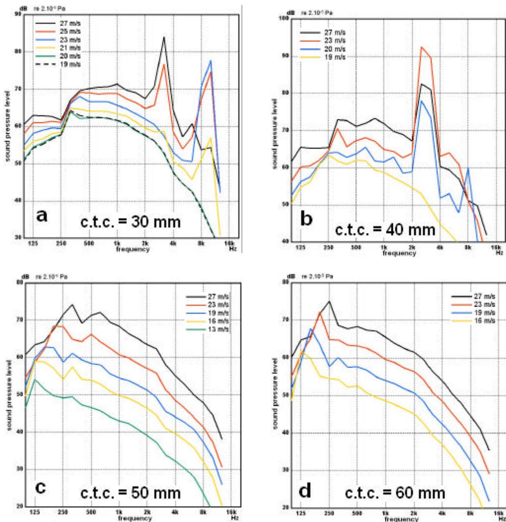
Figure 10a-d: Measurements on the test grating with a bar height of 40 mm.
