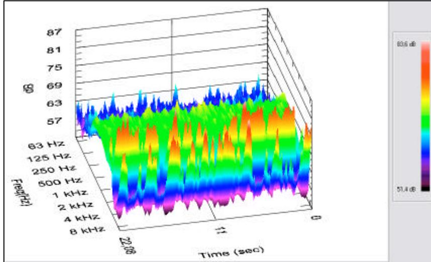
Figure 11: Spectral sound power levels as function of time for grating with bearing bars height / distance of 40 mm / 30 mm at an air velocity of 25 m/s
