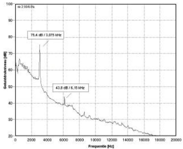
Figure 18a-b: FFT of measurements on the test grating with untreated sharp edges (a) and with tape-rounded edges (b); air flow velocity of 27 m/s.
