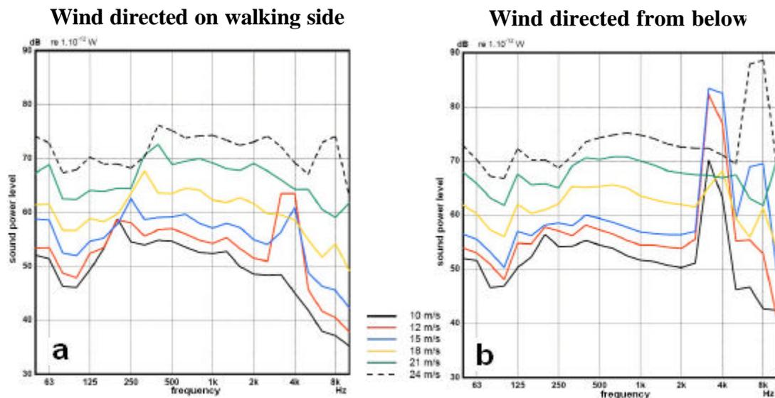
Figure 2: Spectral sound power levels of the grating at different air velocities
