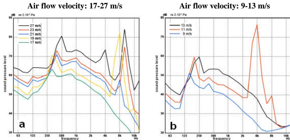
Figure 12a-b: Measurements on the test grating with a bar height of 30 mm and a c.t.c. spacing of 30 mm.
