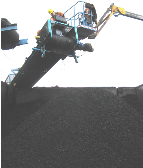
Figure 2: Microphone and measurement system location on top of conveyor belt
