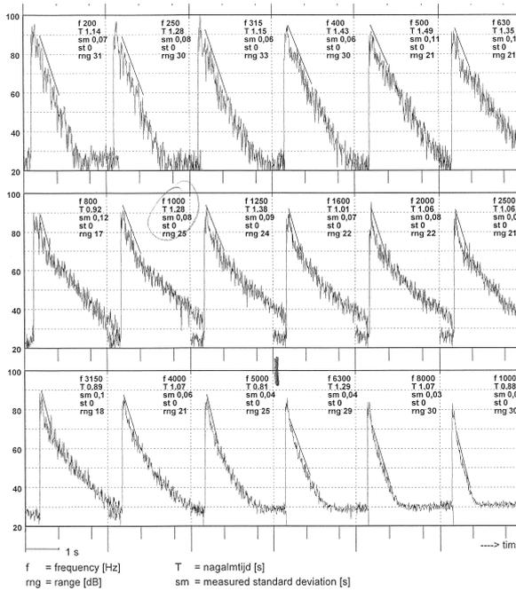
**Figure 1:** Decay curves in third octave bands; some are non-linear
