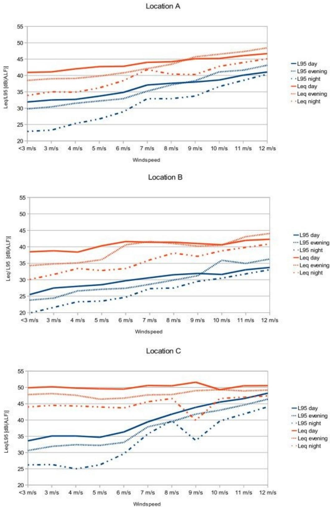
Figure 5 – Measured  $L_{95}$  and  $L_{eq}$  in dB(A,LF) plotted against wind-speed
