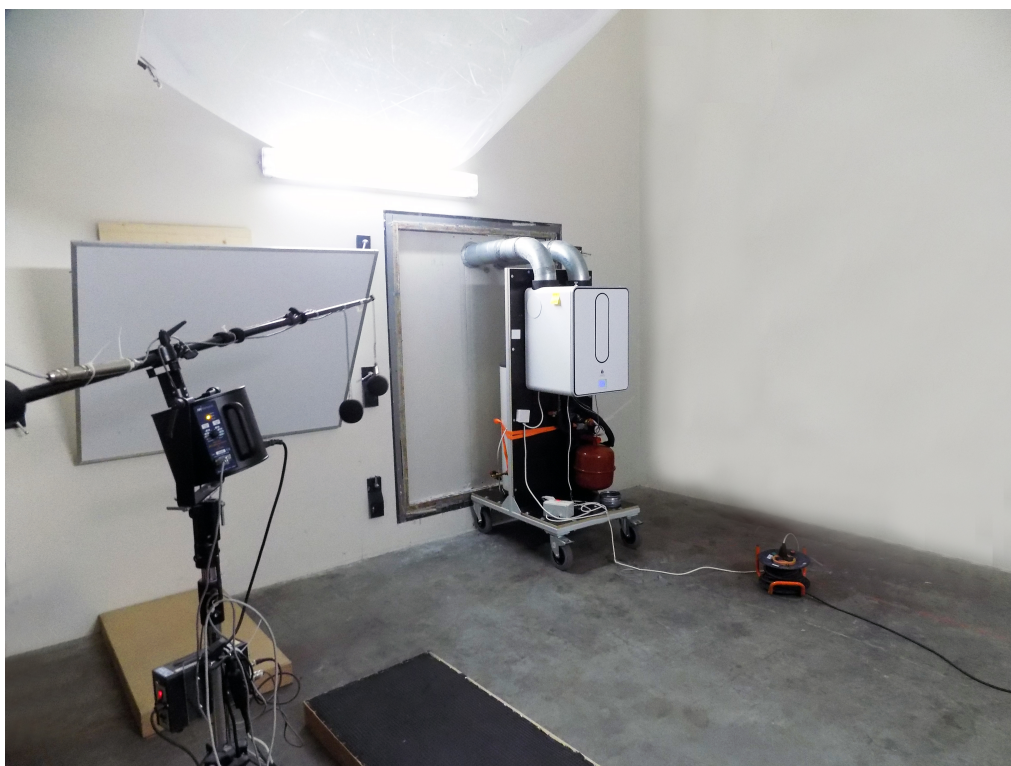
Sound test in our Laboratory for Acoustics
