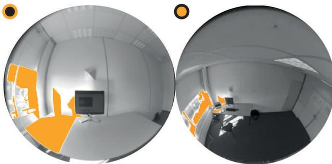
**Figure 8.10:** Glare source areas, indicated in orange, measured at 15:15 on Mar 23 for the benchmark and alternative model.
